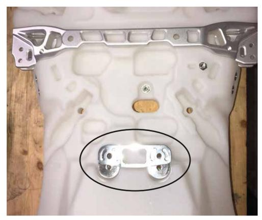
3. ALLIGN BACKPLATE AND APPLY LOCKTITE TO THE TWO M8x25MM FLANGED BUTTON HEAD BOLTS AND INSTALL THROUGH BACKPLATE AND SPACER.
