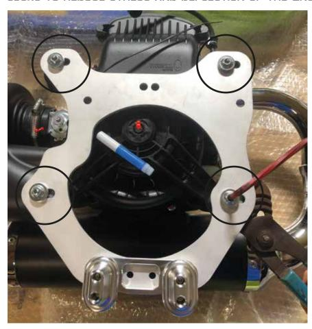
7. PLACE TOWER ON TOP OF THE ENGINE.
